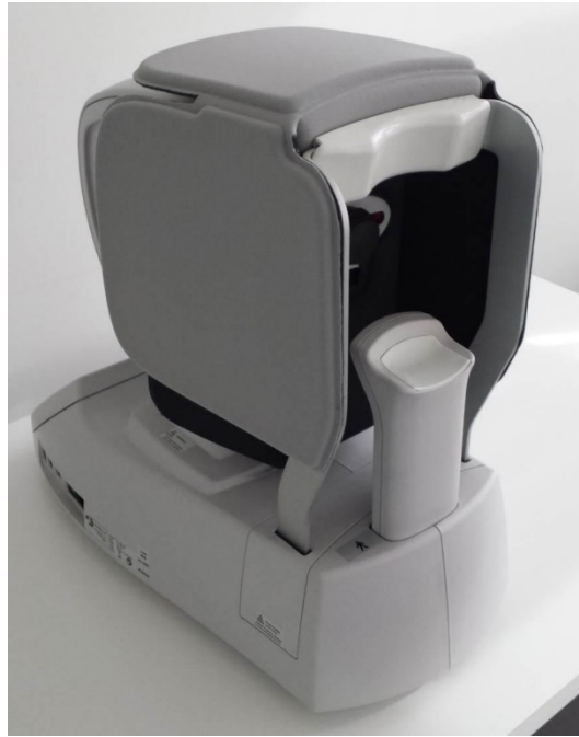
Fig. 3 - Removable light shield or 'hood'
